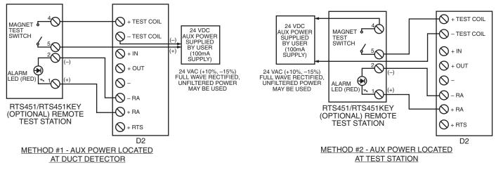
NOTE: THE USE OF EITHER THE RTS451 OR RTS451KEY REQUIRES THE INSTALLATION OF AN ACCESSORY COIL, DCOIL, SOLD SEPARATELY. SEE FIGURE 9 ABOVE FOR REFERENCE.
