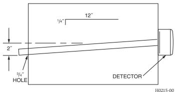
NOTE: Air currents inside the duct may cause excessive vibration, especially when the longer sampling tubes are used. In these cases, a 3 inch floor flange (available at most plumbing supply stores) may be used to fasten the sampling tube to the other side of the duct. When using the flange/connector mounting technique, drill a 1 to  $1^{1}/_{4}$  inch hole where the flange will be used.
