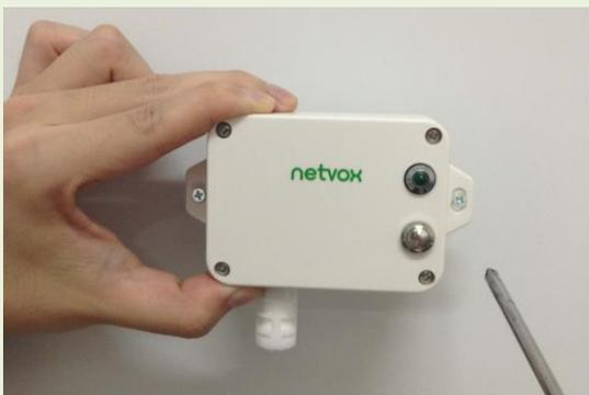
2. When the temperature and humidity detected by R718A is compared with the last reported values, when the temperature change is exceeded 1°C (default) or the humidity change is exceeded 1%(default),it will report current values.
