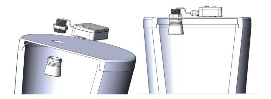
5. If the top of the water tank cannot be opened, the hole made on the top of the water tank is recommended to be 45mm diameter.
