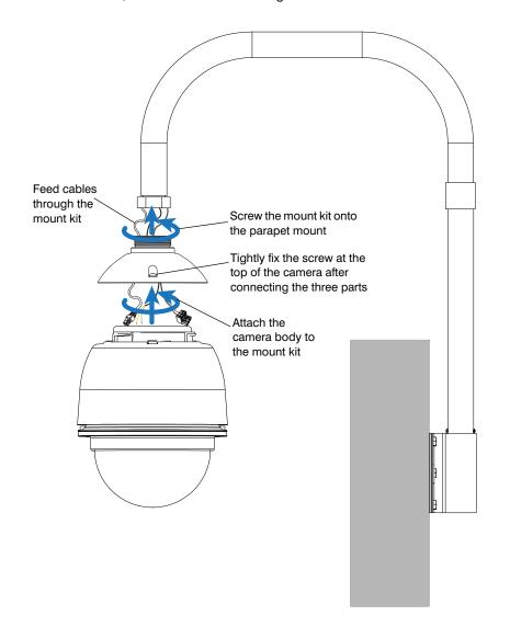
**Note** Check that the eyelet cable connection is secure and carrying all of the load of the camera after making all cable connections.
