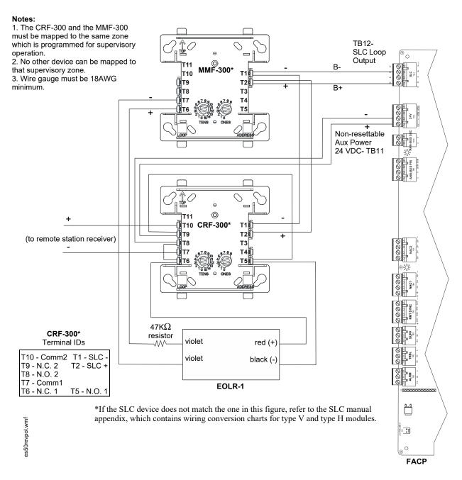
Figure J.3 Alternate Transmission for Supervisory Signals
