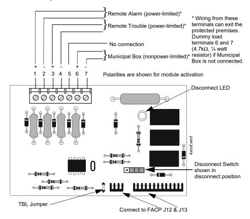
Figure 2.15 4XTMF Transmitter Module
