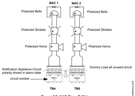
Figure 2.7 NAC Class B Wiring
