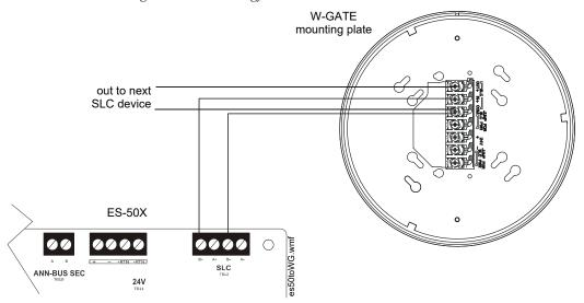
Figure 2.30 W-GATE SLC Connection
