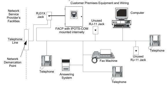
Figure 2.11 Communicator Installation
