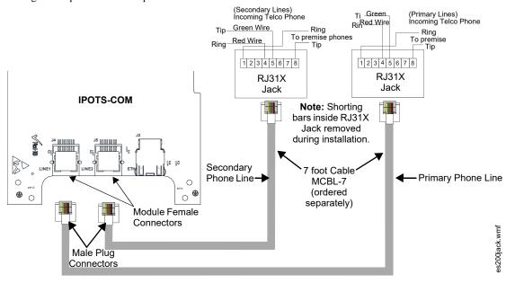
Figure 2.12 Wiring Phone Jacks
