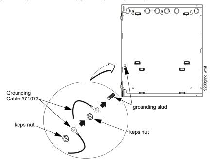
Figure 2.4 Earth Ground Connection
