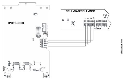
Figure 2.14 Wiring the CELL-CAB/CELL-MOD
