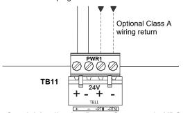
Figure 2.5 Special Application Power Outputs - 24 VDC
