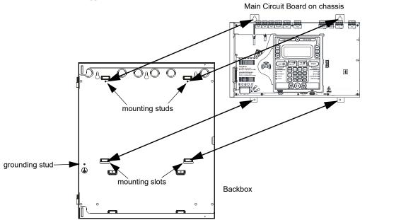
Figure 2.1 ES-50X Chassis Removal and Installation
