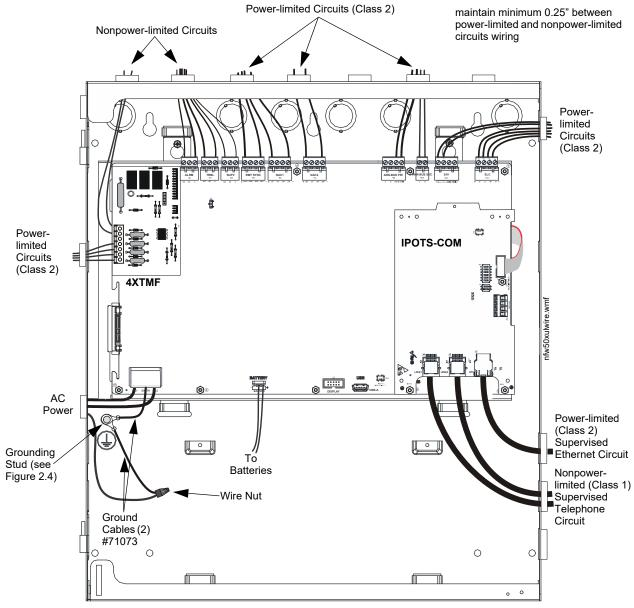
Figure 2.10 Typical UL Power-limited Wiring Requirements
