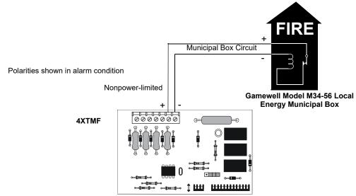
Figure C.1 Municipal Box Connected to 4XTMF Transmitter Module
