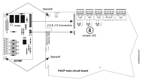
Figure 2.16 4XTMF Connectors to ES-50X Connectors
