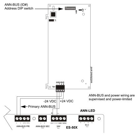
Figure 2.27 ANN-LED Board Layout and Connection to FACP
