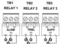
Relay contacts shown <u>with</u> power applied to panel and no active troubles, alarms or supervisories
