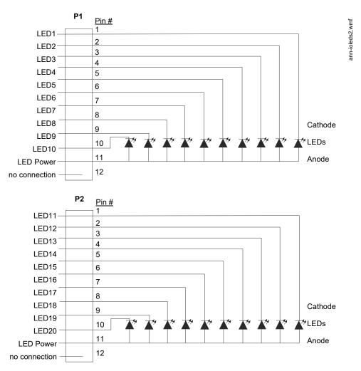
Figure 2.24 ANN-I/O LED Wiring
