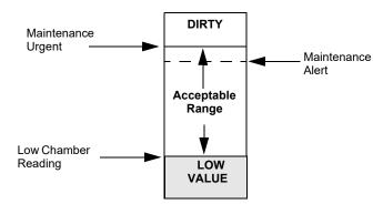
Figure 4.1 Diagram of Maintenance Levels
