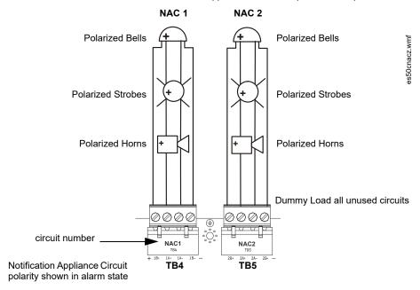
Figure 2.8 NAC Class A Wiring
