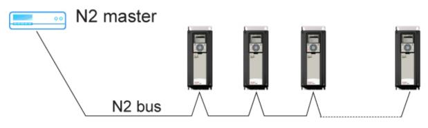
Figure 4. Principal example diagram of Metasys N2
