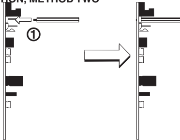
FIGURE 6A: INSTALLATION OF CMF-300-6 MODULE IN A REAR CHASSIS POSITION, METHOD TWO
