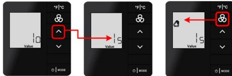
Press FAN button to store the new value. Cloud/Sun symbol blinks to indicate the change in the registry value.
