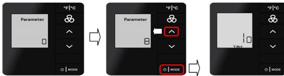
Use UP button to set parameter value to 8 , then press MODE button to view the value
