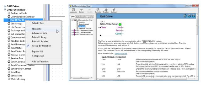
The "DALI F26x Driver" FBox library comprises not only FBoxes to control all parameters and associated devices on a DALI line, but also FBoxes for the configuration and commissioning of DALI devices. This means that commissioning them does not require any external PC software or gateways.
