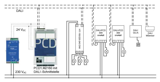
The sample project was wired and prepared according to the above drawing. Please follow the operating instructions for individual components.
