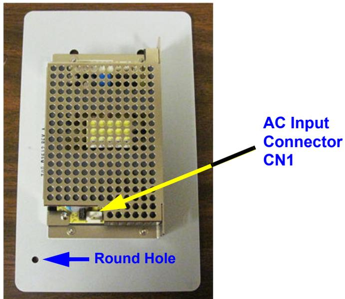
7. Slide the power supply down in the keyholes until they bottom out. Then, tighten the four mounting screws to secure the power supply to the metal plate.
