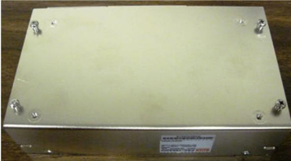
6. Position the power supply over the 4 keyholes on the metal plate making sure that the round hole (see the below figure) is in the bottom left corner as shown and the power supply is positioned with the AC input terminals (CN1) facing downward.
