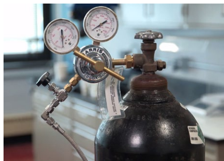
A two-stage nitrogen regulator is required.
