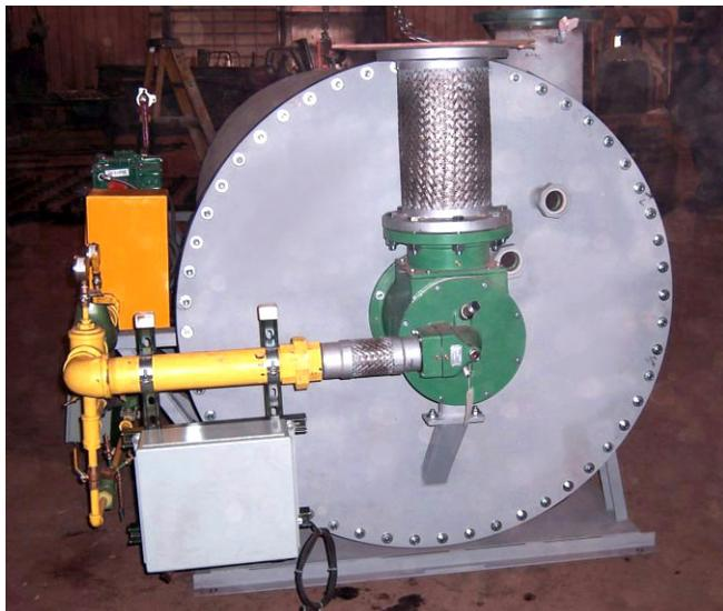
*ThermJet Burner mounted on limestone heater*
