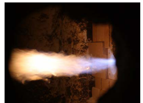
OXY-THERM ® LE staged flame pattern
