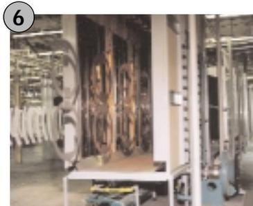
**Photo 5** Air side of pre-mix system for IR burners.
