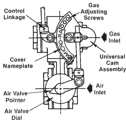
Continue opening the MICRO-RATIO® air valve while watching the manometer connected into the burner's air/gas mixture manifold. Determine the point at which further opening of the air valve gives no appreciable increase in air pressure within the manifold/burner. Mark the air valve dial at this position opposite the air valve pointer. This point will become the maximum air setting for your MICRO-RATIO® Valve mixing tube system.
