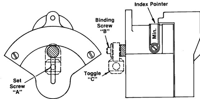
Loosen Allen set screw "A" and binding screw "B" in toggle "C". Move the toggle in universal cam assembly slot towards the center of rotation so that gas valve can rotate from its minimum to maximum position, while the air valve swings between the established (and marked) minimum and maximum settings.
