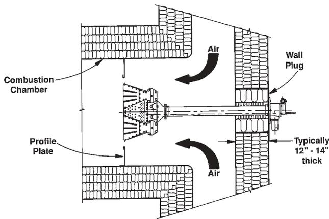
A typical method of through-wall mounting of INCINO-PAK® Burner is shown above. The INCINO-PAK® Burner's back housing is normally mounted and secured onto a separate "wall plug" that is large enough to allow the burner element to be inserted through the duct/chamber wall opening and center itself in the profile plate. The burner element's weight must be independently supported.
