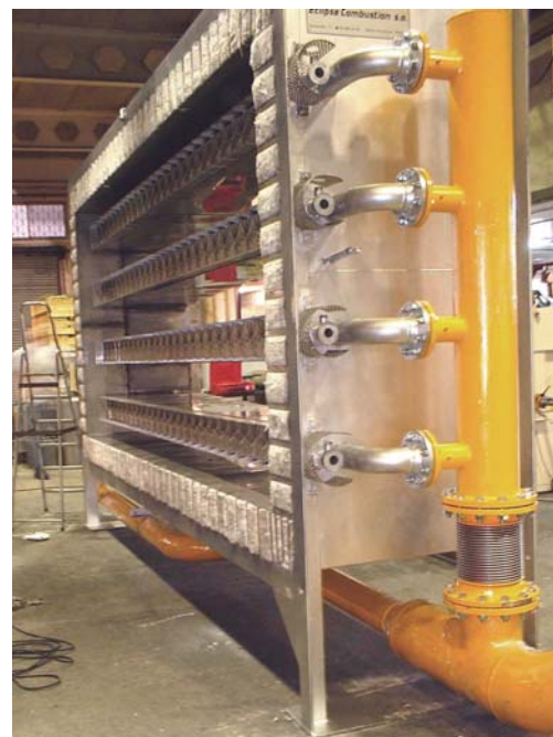
Duct Burner prior to installation showing 4 rows of burner with supplemental air ducting.
