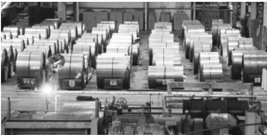
*High temperature annealing is critical to the quality and performance of cold rolled motor lamination steel, used to manufacture transformers, electric motors and lighting ballasts.*
