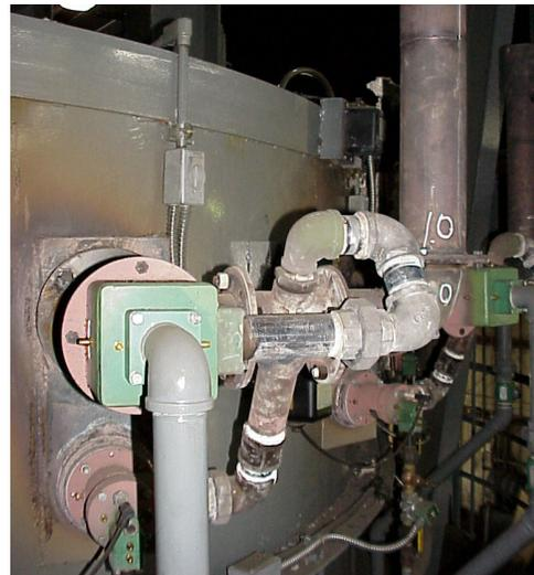
The South Coast Air Quality Management Department (AQMD) in California required that the total NOx production not be increased. The TFB075 burners alone were emitting around 75 ppm @ 3% O<sub>2</sub> (.091 lb/MMBtu) or .47 lb/hr NOx. The TFB burners with recuperators and FGR devices produced 45ppm @ 3% O<sub>2</sub> (.055 lb/MMBtu) or .40 lb/hr NOx.
