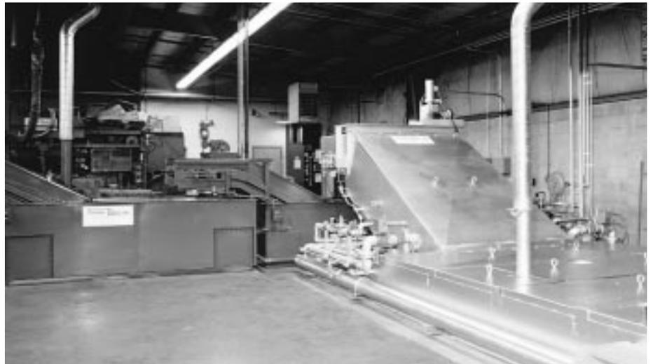
Eclipse Veri-Flame burner controls and other diagnostic components. A TBI semi-closed loop cooling system helps keep fans, hot pulley bearings, and cooling jackets cool utilizing a non-toxic coolant.
