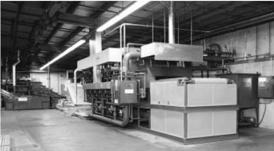
*The austempering line at Eastern Metal Treating is a four-stage process. Parts are heat treated in 3-zone 1500° F hardening furnace, quenched to one desired hardness in a molten salt bath, desalinized in a cold water washer, and desalinized and rust treated in a final hot water washer.*
