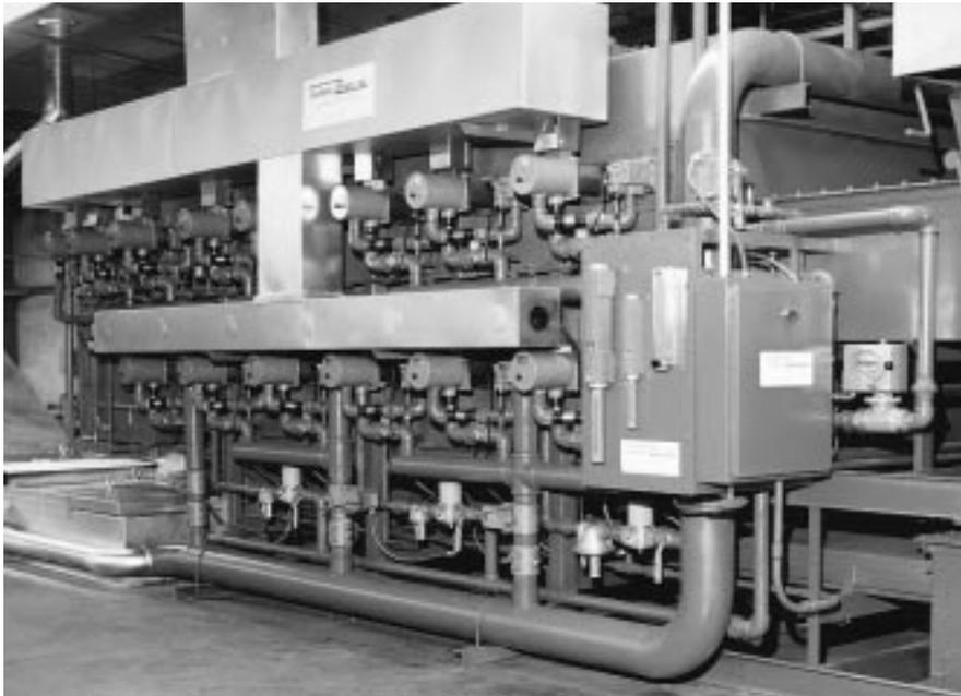
*In the first stage, parts are conveyed into the 3-zone 1500° F hardening furnace heated by 14 Eclipse ThermThief (Model 30 TFB) burners firing horizontally into radiant tubes equipped with Bayonet-Ultra recuperators at 3,000,000 BTU/hr.*
