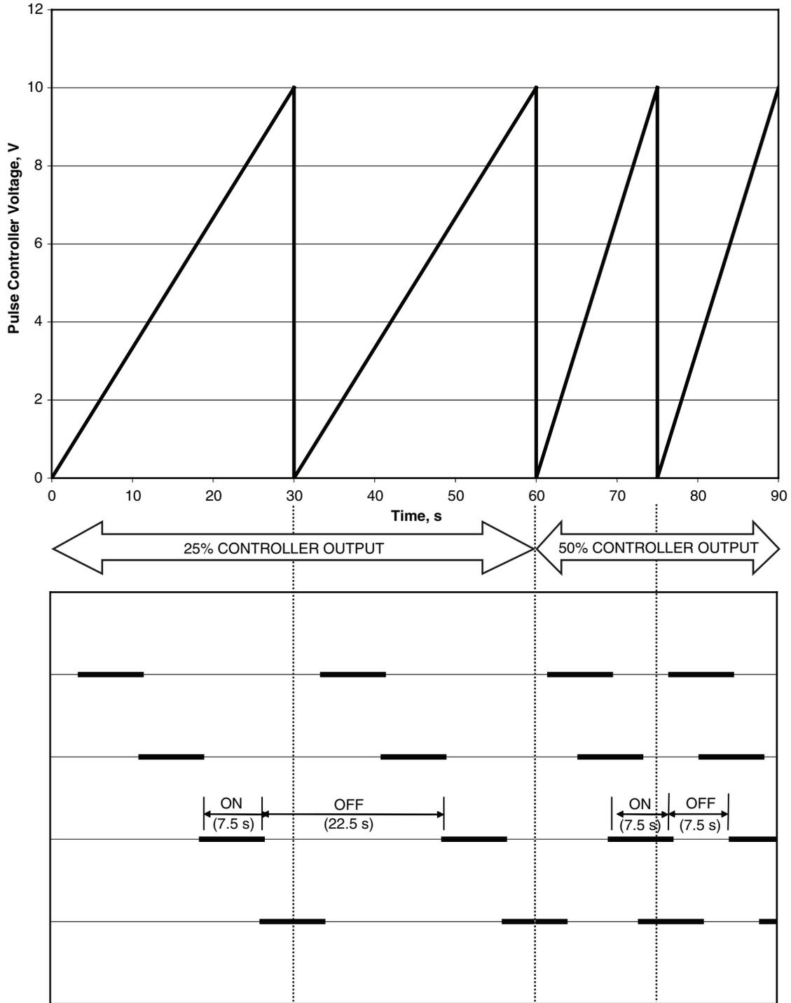
Figure 7: Four-burner system with the burner firing sequences for 50% and 25% output
