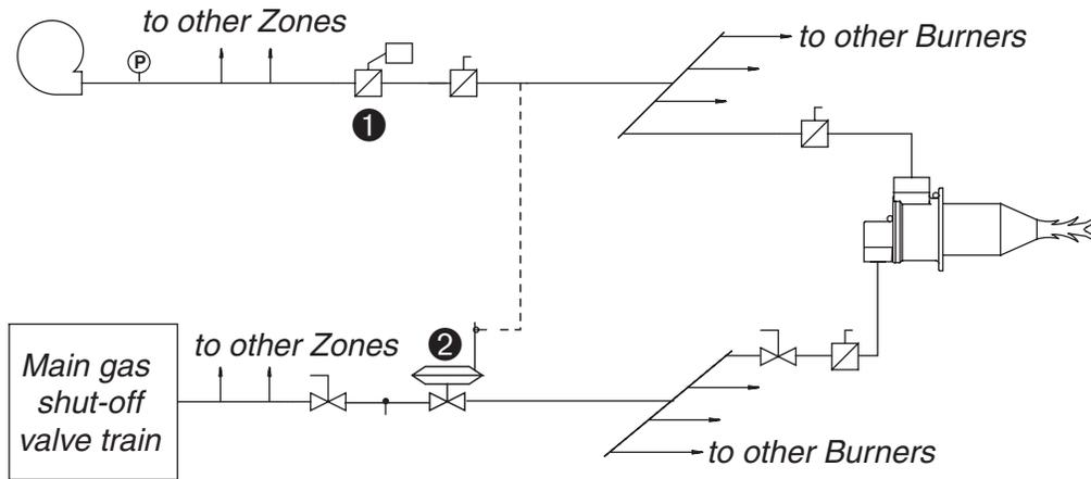
Figure 1: Typical amplitude-modulated combustion system
