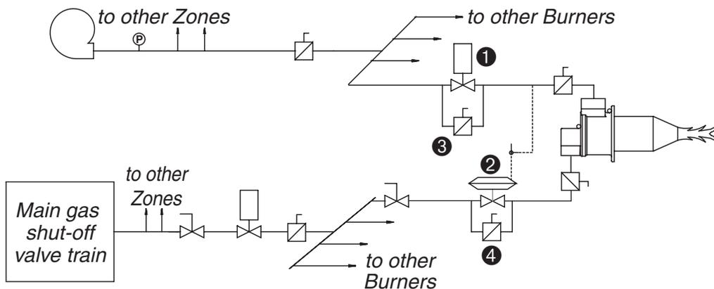
Figure 2: Typical high-low frequency-modulated combustion system
