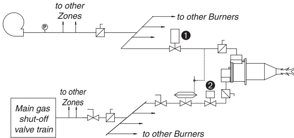
Figure 3: Typical on-off frequency-modulated combustion system
