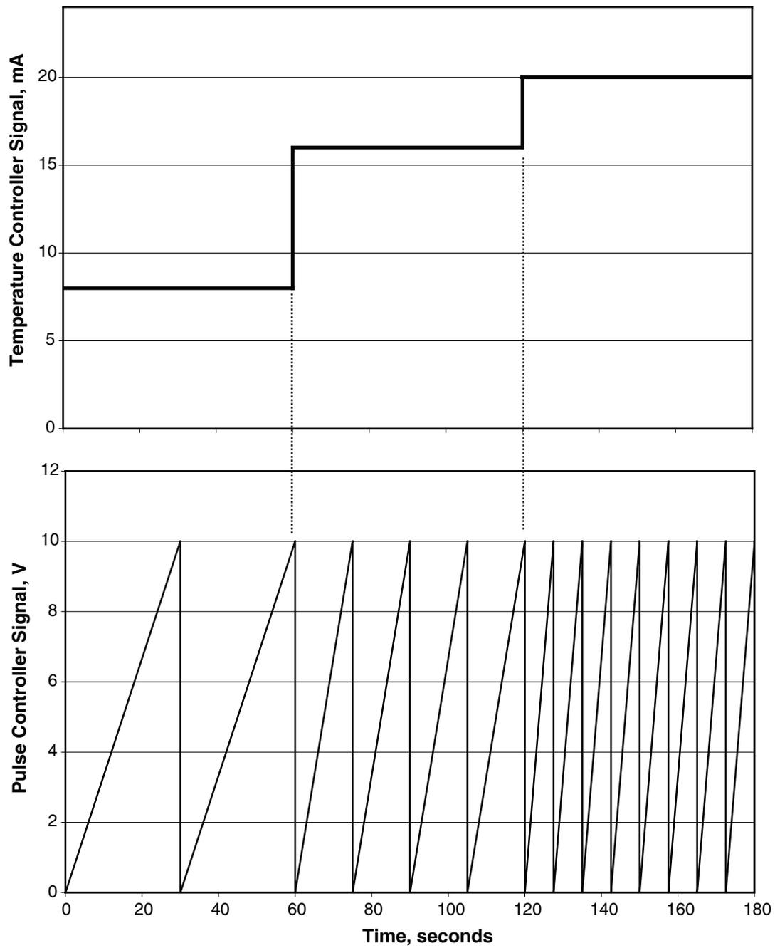
*Figure 4: Temperature controller signal conversion*
