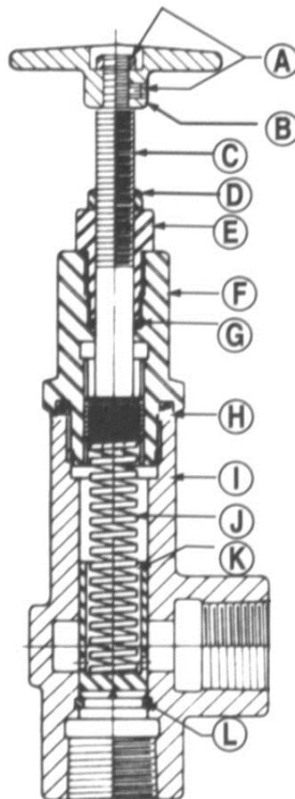
Figure 5. Cross-Sectional View of a Pressure Relief Valve
