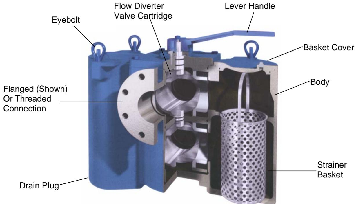
**Figure 4. Cutaway View of Double Basket Strainer**
