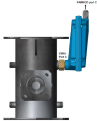
Fig. 4. Heat exchanger mounting example with vertical mixing unit orientation (shown with 300kW Mixing Unit)
