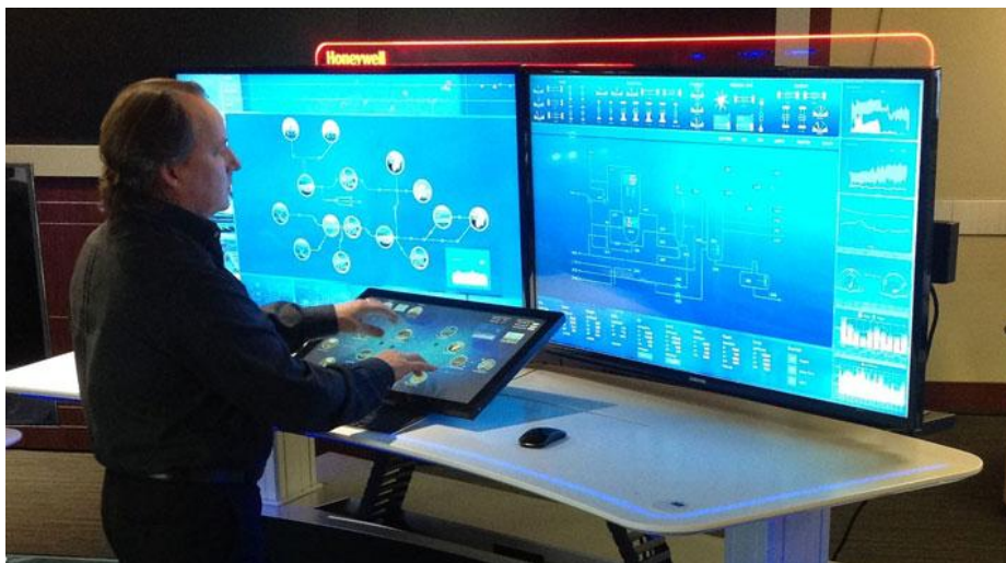
Figure 5. The Experion Orion Console is designed to help operators solve process issues while working on a platform that allows them to stay mobile.
