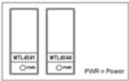
Figure 22.6 Analog Input - MTL4541 and MTL4544 isolator LED indicators
