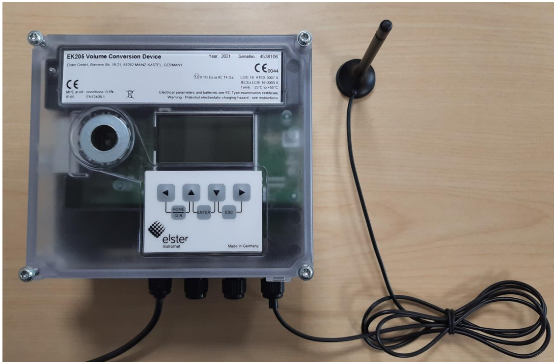
Fig. 35: EK205-M with external antenna installed
