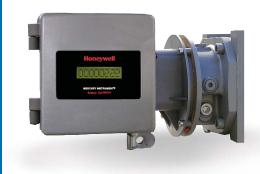
This direct-mount electronic volume corrector is available for most popular rotary gas meters. The internal temperature probe and independent Redundant Electronic Index (REI) improve the precision and reliability. The Mini-Max Rotary Corrector easily adaptes to Dresser LMMA & B3, Romet and Elster American Meter\* B & C-body rotary meters.
