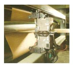
Scanning coat weight sensor
