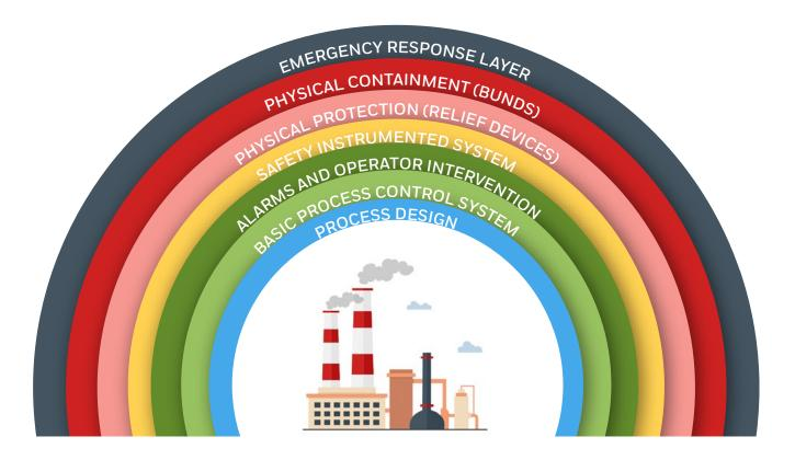
Layer of protection analysis (LOPA) is a risk management technique commonly used in critical process industry such as refineries, chemicals etc. that can provide a more detailed assessment of the risks and layers of protection associated with hazard scenarios. By using the LOPA method, the user is able to ascertain the level of risk that is associated with hazardous events in the workplace.
