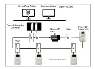
Figure 8: Native integration of Honeywell VFD
