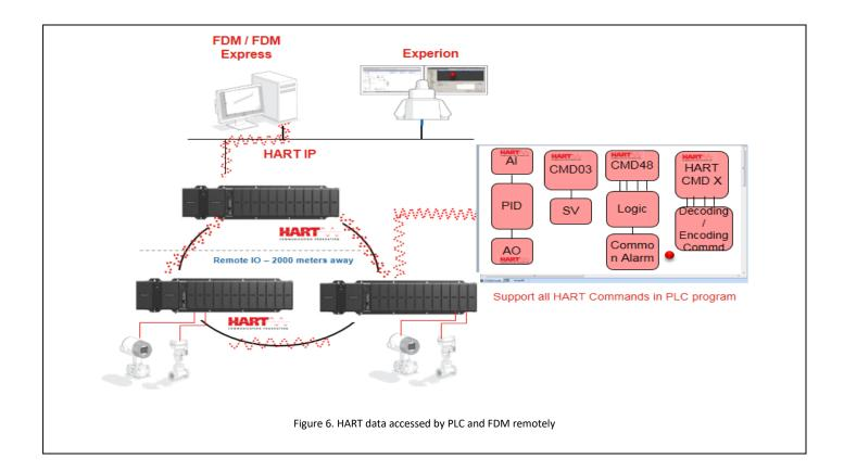
the HART-IP open standard and investment protection through the use of existing plant network infrastructure. Finally, FDM conveniently co-exists on the ControlEdge Builder workstation and is scalable to large sized projects.
