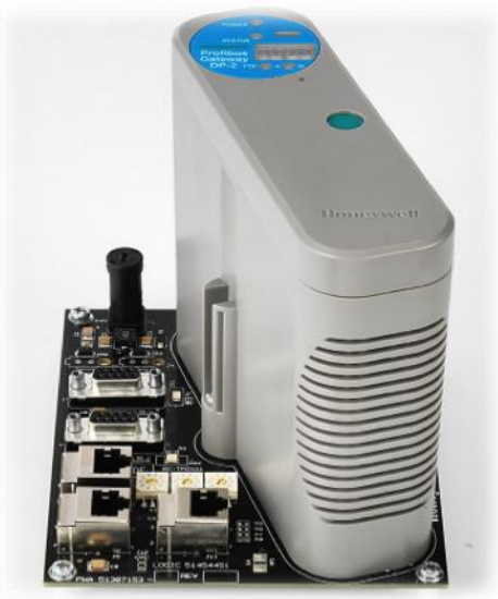
Figure 3. Honeywell's robust Experion C300 controller.
