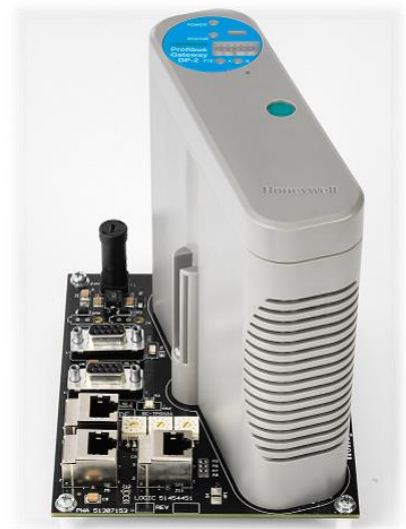
Honeywell's robust Experion S8 C300 controller
