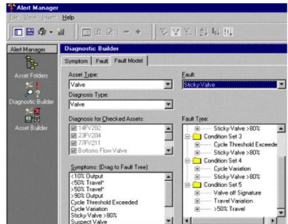
Alert Manager provides simple diagnostic configuration with easy drag and drop capabilities to quickly build fault models.
