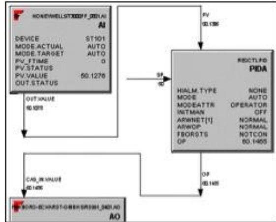
Connections between fieldbus and controller blocks are easy with the Experion Control Builder tool.
