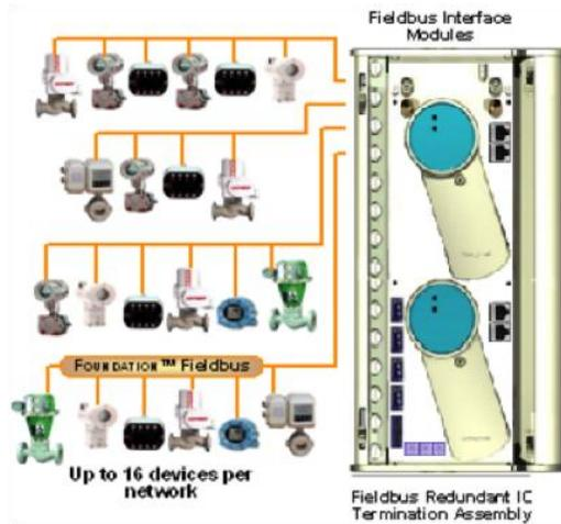
With PlantCruise by Experion, your fieldbus system is secure. A redundant FIM4 is shown above.
