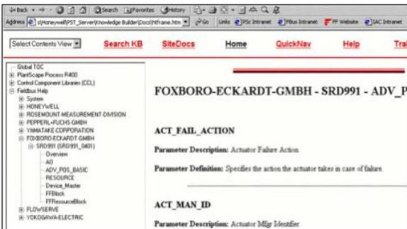
Help information from DD files is automatically added to Knowledge Builder and indexed to Control Builder.
