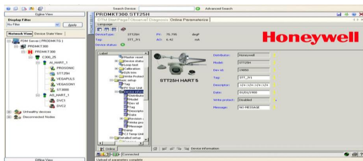
FDM used for Honeywell STT25H Temperature Transmitter
