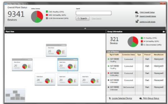
Figure 4. Field Device Manager Plant Area View
