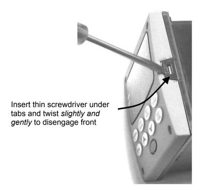
Using a thin screwdriver, *gently* twist the screwdriver to pry the side tabs from the front face. Pry just enough to release it, *otherwise you'll bend or break the tab*. If you break or bend the tab and can't reattach the front snugly, you'll need to reattach the front using the 4 NEMA4 screws provided.
