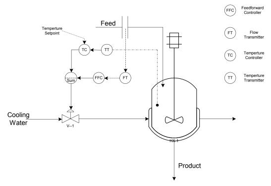
Feedforward control on the feed to a continuously stirred tank reactor operating under reactor temperture control
