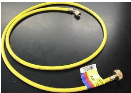
A liquid discharge line with a CGA-660 connection and gasket is required
