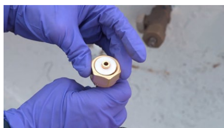
In North America, a liquid discharge line with a CGA-660 connection and gasket is required.
