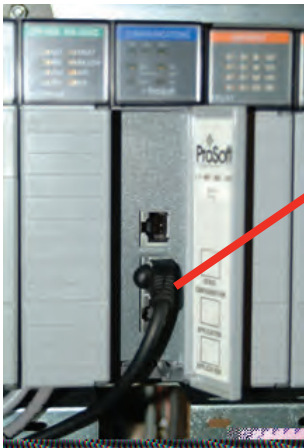
Figure A-4. DF1 Connection to RJ45 Socket
