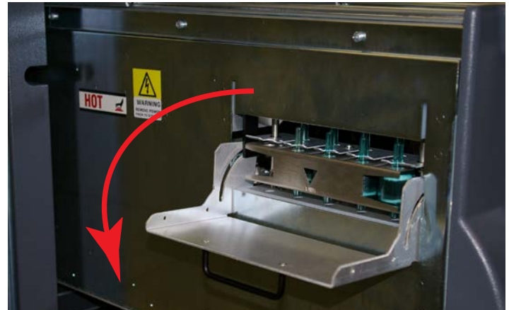
Figure 5-5. Pyrolyzer Filter Door
