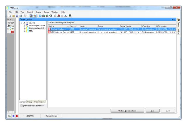
Please check if the DTM revision number (Device version) mentioned in the device catalog corresponds to the device revision number of the physical Optima Plus device you intend to connect.
