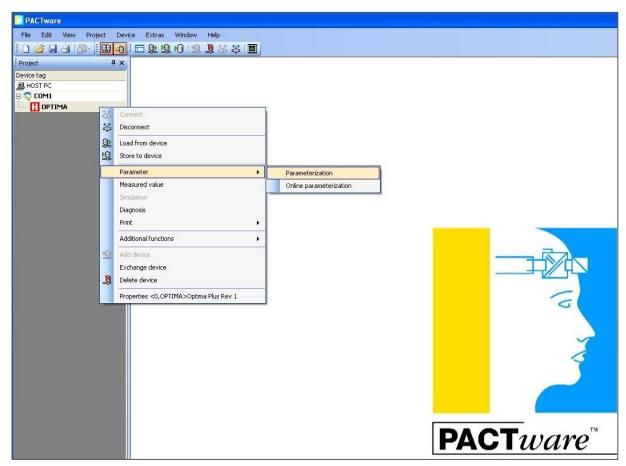
Offline configuration is the ability to manipulate device parameters without the presence of a physically connected device (commissioning, device exchange, device data set archiving). Offline parameters are stored by the FDT frame.
