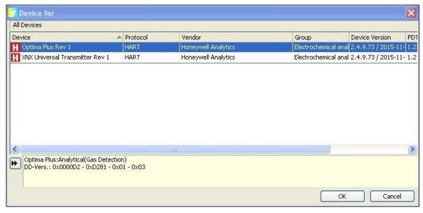
11. Go online by right-clicking on the device DTM and select "Connect" to connect the Optima Plus device:
