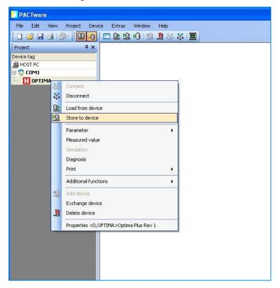
To store parameters to the device, the Level2 password must be entered.
