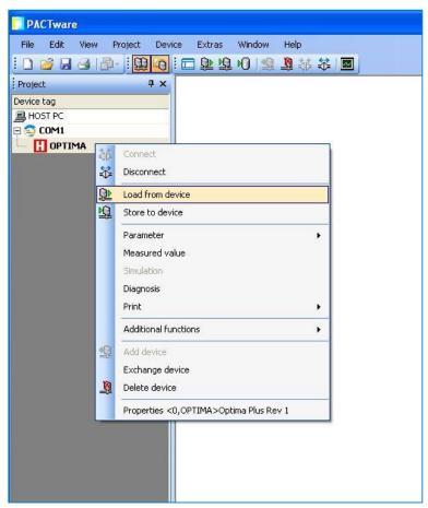
After clicking "Load from device" icon, an "Upload" screen will be shown and the upload progress bar. When the progress bar is through building, you can click on the "Edit device parameter" icon.
