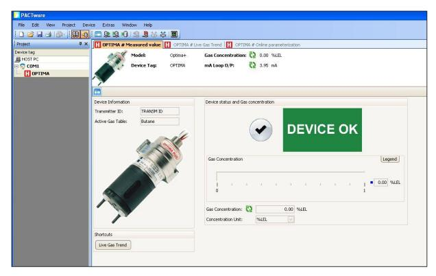
Device status display. The following states of the Optima Plus in order of increasing severity can be shown in this area:
