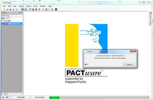
14. Once data upload is completed, the device name is changed to the device tag as below. Then double click the device tag or click 'Parameter\Online parameterization' from context menu to view online parameter.
