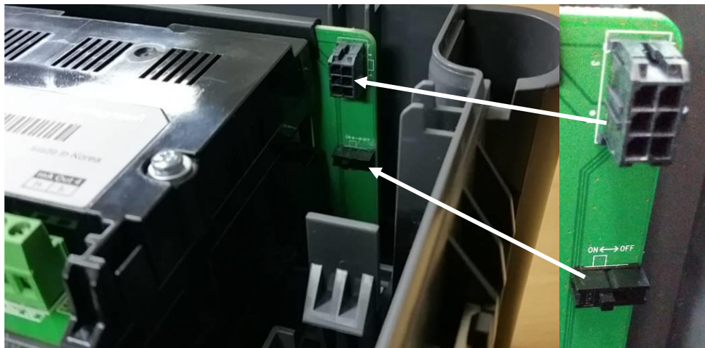
Figure 12. Battery On/Off Switch and Battery Connector
