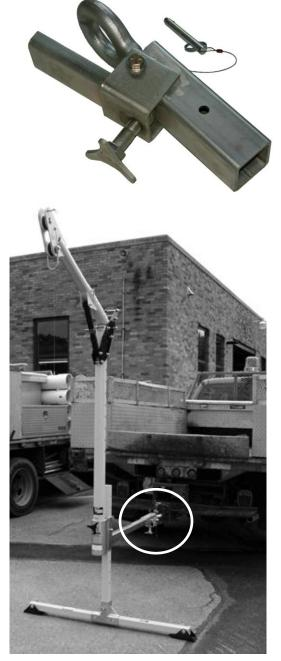
Pintle Hitch Adapter installed between the DH-12 and vehicle.
