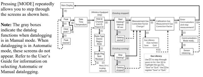
**Note:** The gray boxes indicate the datalog functions when datalogging is in Manual mode. When datalogging is in Automatic mode, these screens do not appear. Refer to the User's Guide for information on selecting Automatic or Manual datalogging.
