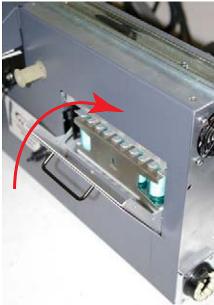
Analyzer Filter Door
