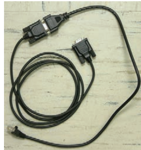
Figure F-5 -- Debugging Cable
