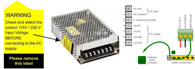
Figure 4. Switched Mode Power Supply (SMPS) Connections
