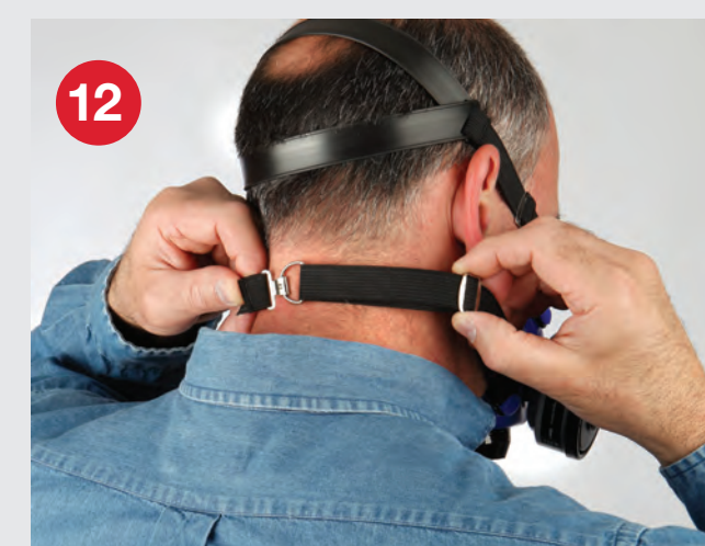
Tighten the lower head straps by pulling evenly on the end straps in the back of the respirator until the entire respirator is snug, comfortable and centered on your face.
