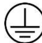
Figure 4. Equipment Earth (Ground) Point
