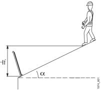
Each Class is recommended for use with a range of roof slopes and potential fall heights.
