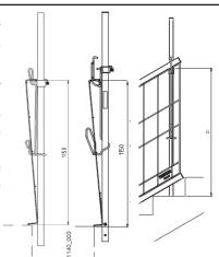
3. The hooks on the Steel Mesh Barrier Holder are to be at right angles to the Cloxy.
