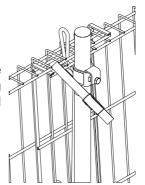
For class C minimum overreach/overlap needs to be two meshes for SMB and one mesh for SMB Lightweight.
