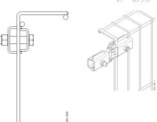
3. Check that the raised surface on the Steel Mesh Barrier Hinge is positioned in between the vertical rods.
