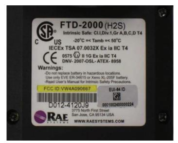
Figure 2: MeshGuard Detector equipment certification label.
